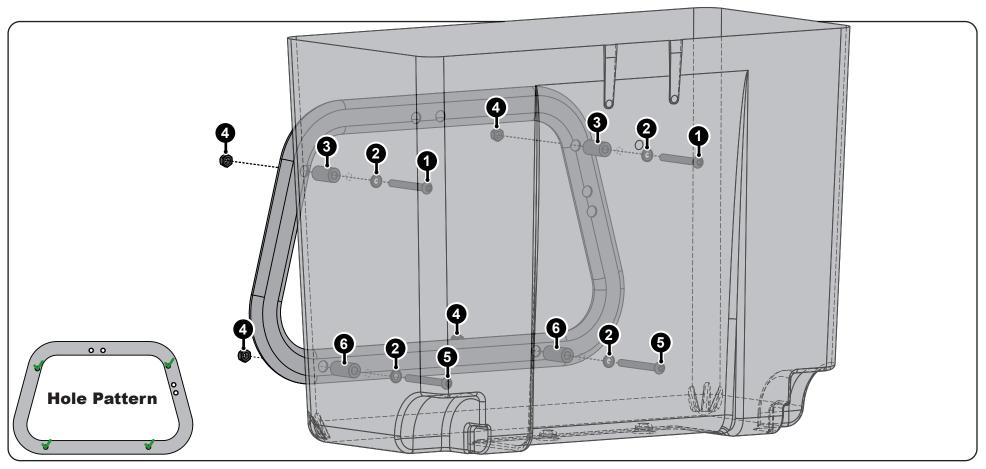
**Step One:** Place the side carrier on the back of the luggage case and mark the hole pattern on the case. Using a 6mm drill bit, drill all four holes through the back side of the case.
