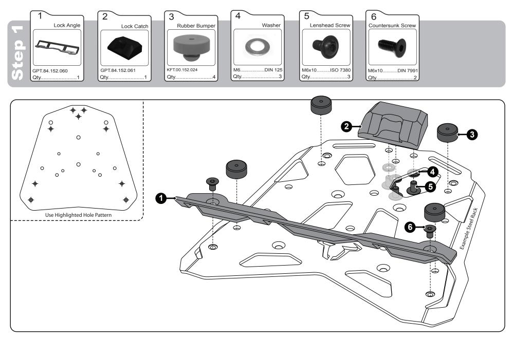
**Step One:** Mount the Lock Catch and Lock Angle to your Steel Rack in the position illustrated above and torque to specs. Next press the rubber bumpers into the Steel Rack in the positions illustrated above.
