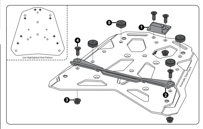
**Step One:** Mount the Lock Catch and Lock Angle to your Steel Rack in the position illustrated above and torque to specs. Next press the rubber bumpers into the Steel Rack in the positions illustrated above.
