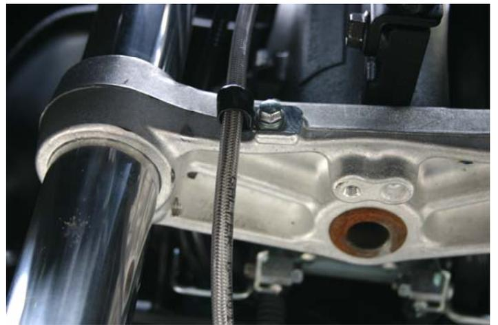
**b. Line A with Galfer c-clip at the lower triple tree**
