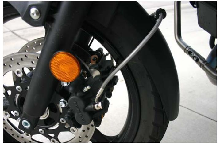
**h. Line C routed over the fender to the left caliper**
