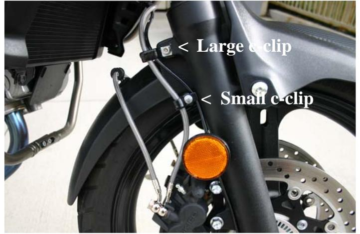
**f. Line B & C at right caliper, notice c-clips at fork**
