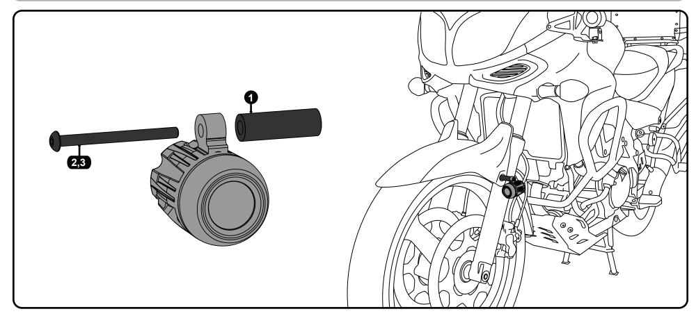
**Step One:** Determine if your motorcycles fender mounts are using M5 or M6 bolts, then assemble the light pod and hardware accordingly. Once assembled bolt the light pod directly to your fenders mounting points.
